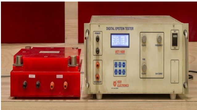
Epstein Bridge tester for testing Core loss of CRGO and CRNGO Electrical steel
