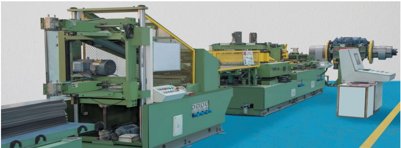
Automatic CNC Cut-to-length machine (up to 440 mm width)
