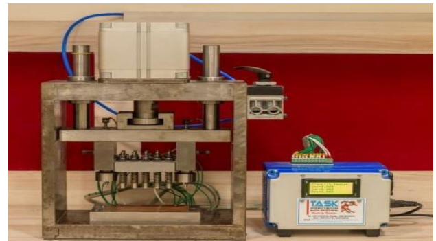
Franklin tester for testing surface insulation resistivity of CRGO Electrical steel
